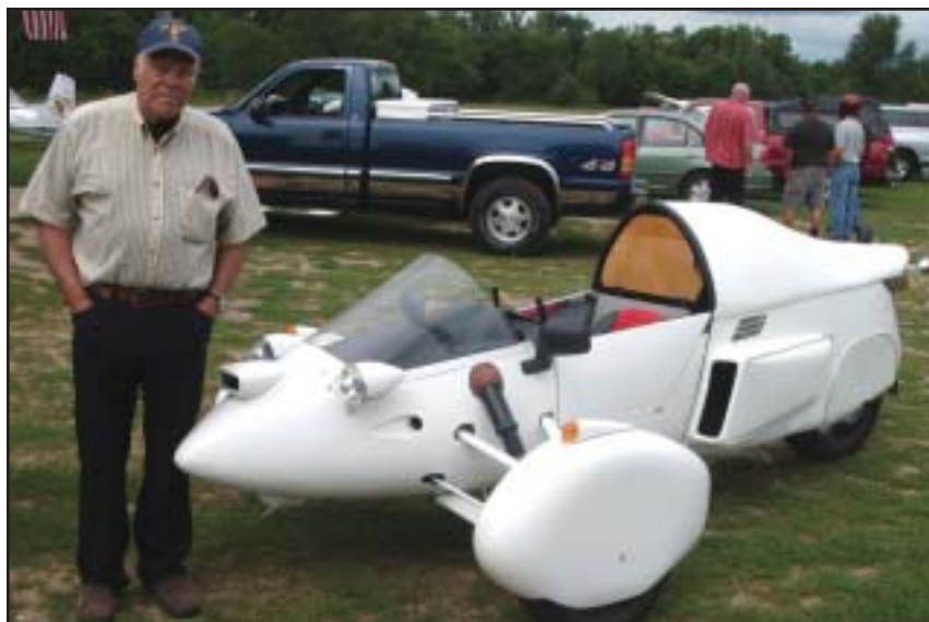
Tim Buttles stands next to his white Aero-Cycle. Under the streamlined body is a complete Honda 600 RR motorcycle.
