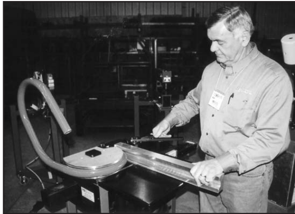
Bill Politsch, of Mittler Bros. Machine & Tool, demos the use of a tubing bender during the Lefthander Chassis trade show. Lefthander sells the Mittler Bros. line of quality metal fabbing tools.
