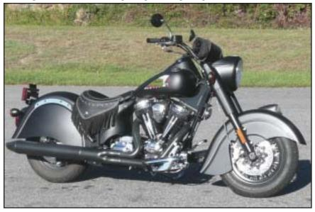
**The Motorcycle**: 2010 Indian Dark Horse, rigid mounted fuel-injected 105 Cubic Inch Power-Plus V-Twin engine, 6-speed Trans, and Brembo disc brakes. It was all stock except for the fringe on the seat – it was the only added option. List base price (from the website): \$27,999.00 plus set-up and taxes.
