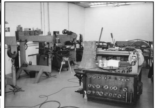
The L'Cars restoration shop, in Cameron, Wis., sometimes uses these giant English wheels to build custom motorcycle tanks. This shop has a metal fabrication how-to video on its Website.
