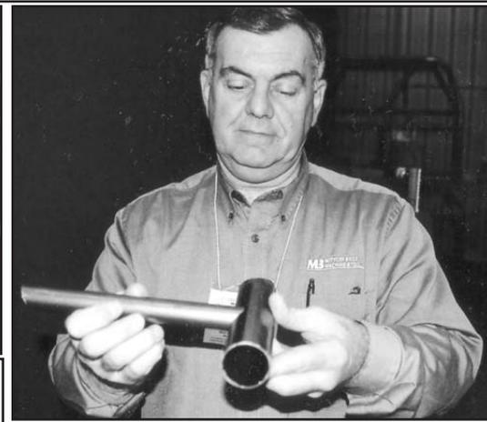
Bill Politsch shows how the notched piece of tubing fits perfectly up against a larger piece of tubing. This type of tool is great for fabricating or repairing motorcycle frames.
