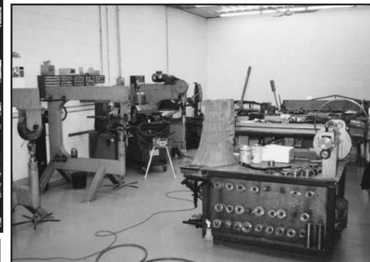
The L'Cars restoration shop, in Cameron, Wis., sometimes uses these giant English wheels to build custom motorcycle tanks. This shop has a metal fabrication how-to video on its Website.
