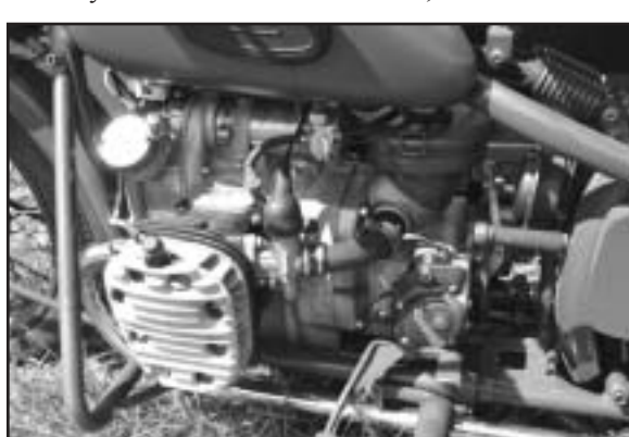
The finned cylinder head is on the side of the engine and crash bars protect the engine in the case of a tip over.
